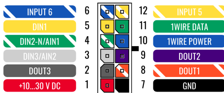
FMC130 2x6 socket pinout
