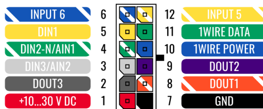
FMC234 2x6 socket pinout
